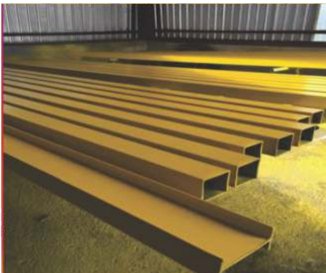
Blasted and painted Structural Members, ready for load-out.
