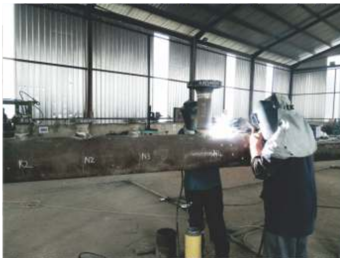
Fabrication of 12 inch & 6 inch Pig launchers & Receivers for Njaba End Facility project.
