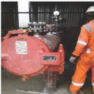
Fabrication of 12 inch & 6 inch Pig launchers & Receivers for Njaba End Facility project.
